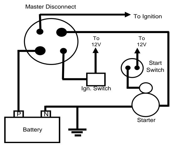
Note: May also run alternator field wire through disconnect switch instead of ignition circuit. Do not run Alternator output through disconnect switch. *WWW. fastroni xsol utions. com*
