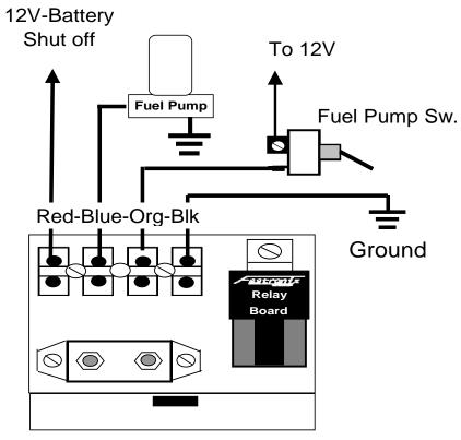
Mount relay board to chassis tubing using included clamp. Strip wires and install under proper terminal screw and tighten. Connect wires per diagram using proper gauge wire for your application.
